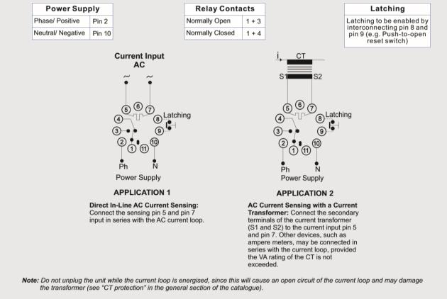
**Detecting Reverse Power:** Ensure that the unit is powered from the same phase as the phase in which the current is being measured. If the "reverse power" LED illuminates under normal operation, it means that the polarity is incorrect and the leads to the current transformer should be exchanged.
