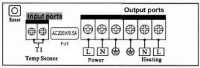
FU1 is the fuse of controller, AC250V/0.5A
