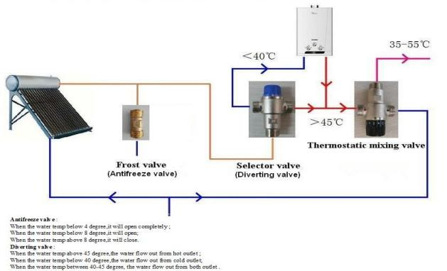
Thermostatic mixing valve : Temp. range is 35-55 degree
